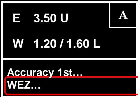
On the main ballistic screen, scroll down until you see WEZ and press the center button.
